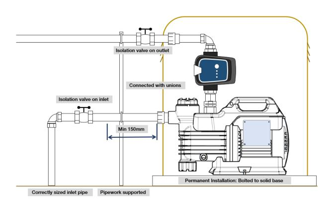
Never run the pump before filling with water.
